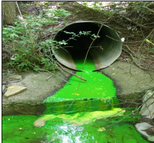
Green dye is added to groundwater to help understand water movement through karst areas common in Kentucky.
